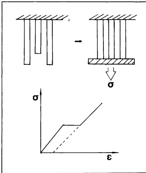
Fig. 8. Simple model for describing apparent plastic deformation arising from residual stress.
