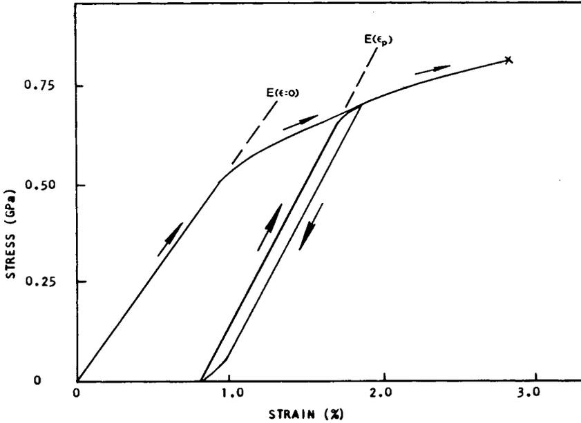
Fig. 7. Stress-strain behavior of as-spun PBT fiber.
