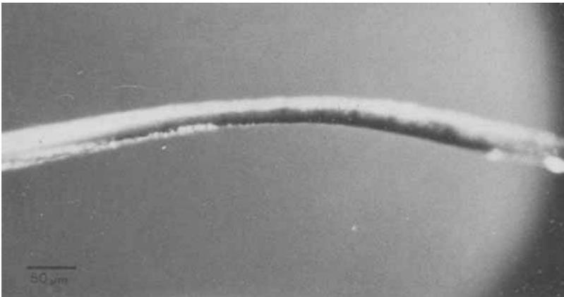
Fig. 10. Optical micrograph of initially straight PBT fiber which was laser burnt. Burnt region is on concave side, suggesting residual compressive surface and tensile core stresses.
