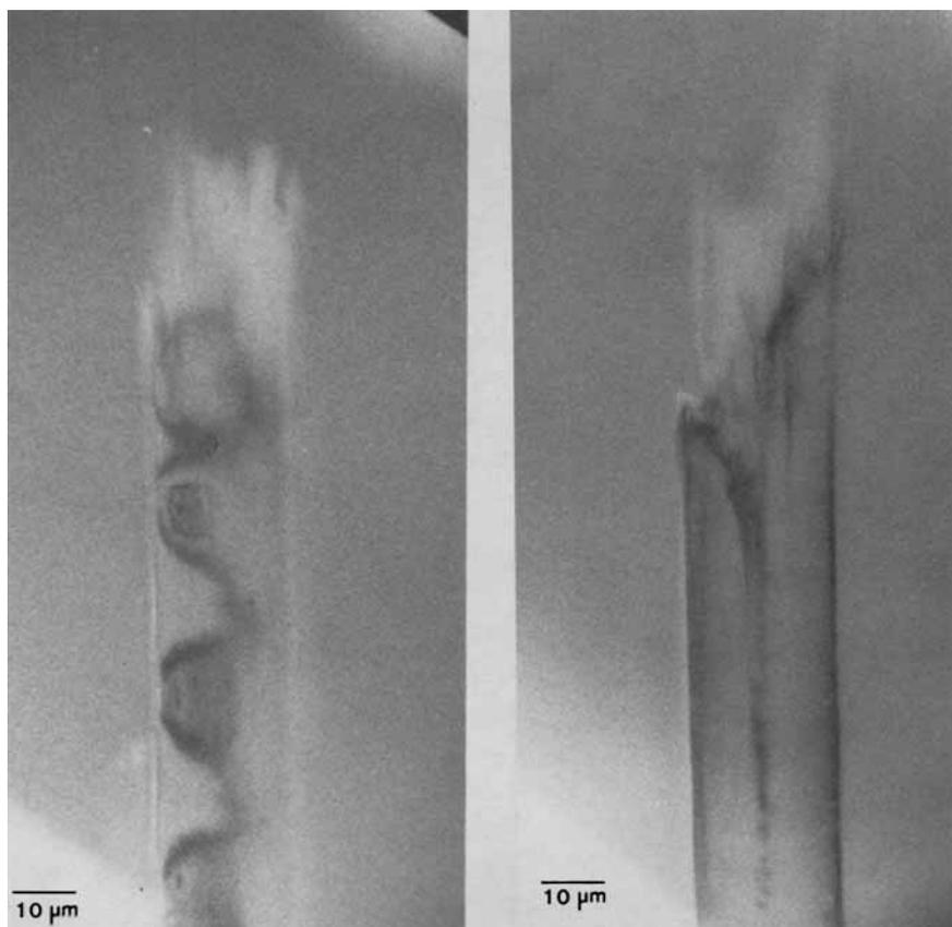
Fig. 3. Optical micrographs revealing void-localized fracture of tensile-tested PBT fibers.
