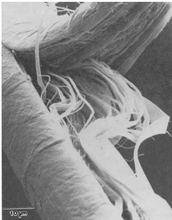
Fig. 1. SEM of PBT fiber peeled to reveal internal fibrillar character.
