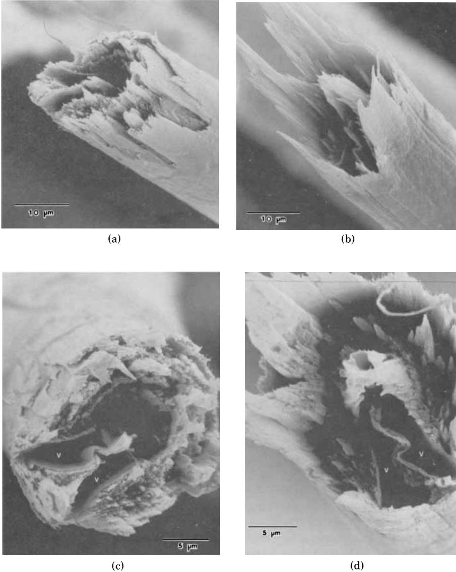
Fig. 4. SEM side views (a),(b) and end-on views (c),(d) of matching fracture ends of tensile-fractured PBT fiber. Elliptically shaped regions in (c) and (d) indicate void (v).
