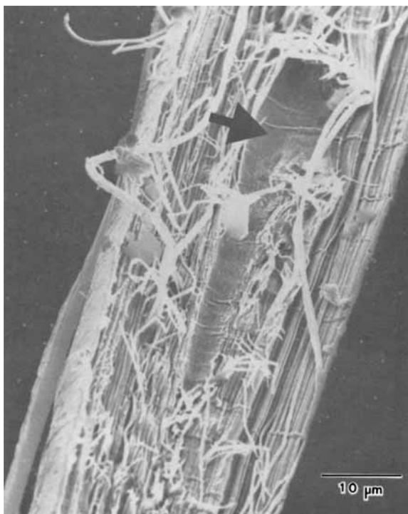
Fig. 5. SEM micrograph peeled PBT fiber revealing presence of void.
