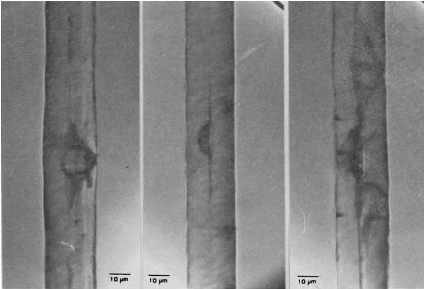
Fig. 2. Optical micrographs of voids in as-spun PBT fibers.
