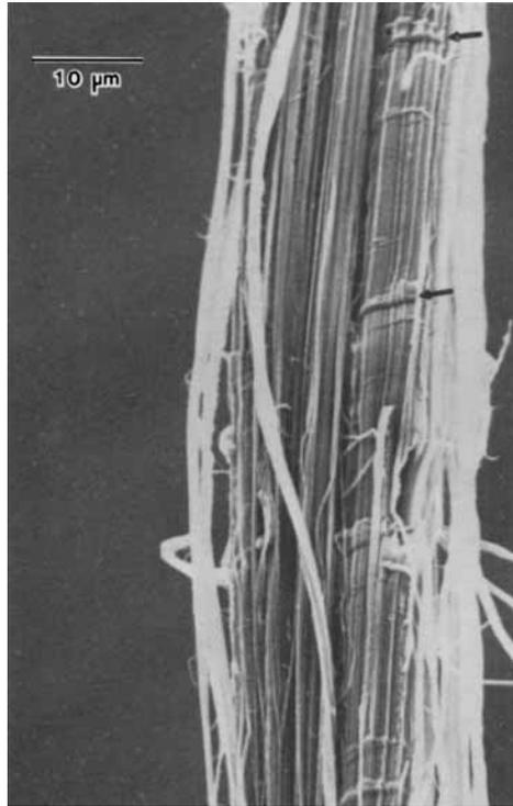
Fig. 6. SEM micrograph of deformation or kink bands (see arrows) in peeled PBT fibers.
