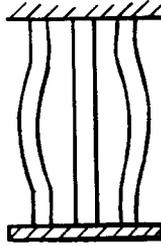
Fig. 9. Residual stress model which incorporates modulus variation with plastic strain.
